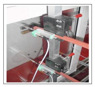
It is also possible to equip the test wall with an add on part to put in a cooling or heating unit. This allows to perform thermal tests.
