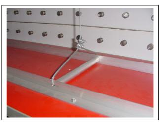
The test wall can be equipped with electronic or mechanic deflection micrometers. The fixing-bar as well as the micrometers can be mounted on each place.
